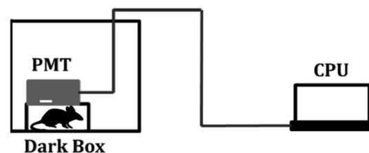
**Figure 1.** Diagram of the experimental arrangement where the photon flux densities within the same space (the small dark rectangle containing the mouse silhouette) was measured. The grey rectangle refers to the PMT and the small thin white rectangle indicates its aperture above the mouse. All of the equipment was placed in a larger box. The computer system recording the data was external.
