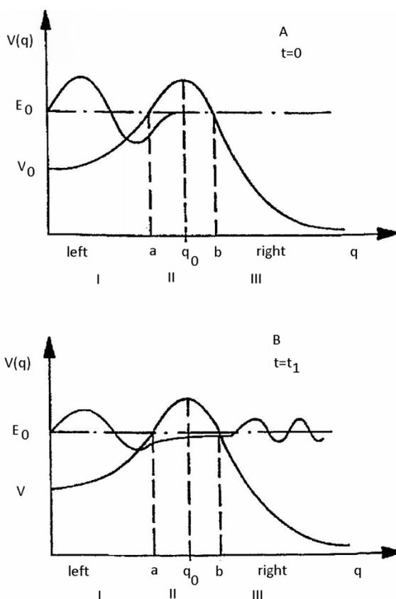
**Figure 7.** (Upper), the initial state ( $t=0$ ) of the quasiparticle in the potential  $V(q)$ . The quasiparticle wave function is located to the left of the barrier.  $E_0$  is the energy of the activated state which starts to tunnel through the barrier. (Lower), after time  $t_1$  the wave function has components on both sides of the barrier.  $a, b$ : classical turning points of the motion inside and outside the barrier (Beck and Eccles, 1992).
