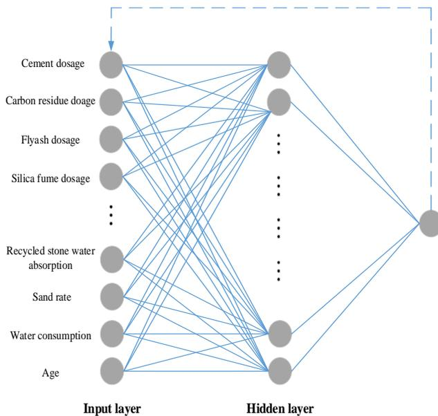
**Figure 2.** Model structure diagram
