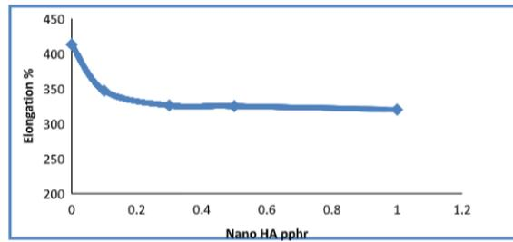
Fig. 7. Impact of nano HA on the elongation of the composites
