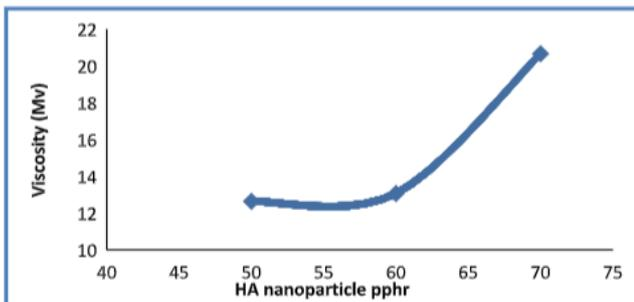
Fig. 4. Effect of HA nanoparticles on the viscosity of RTV-LSR matrix
