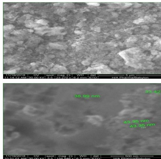
**Figure 2.** The SEM micrograph of the HA/RTVLSR nanocomposites
