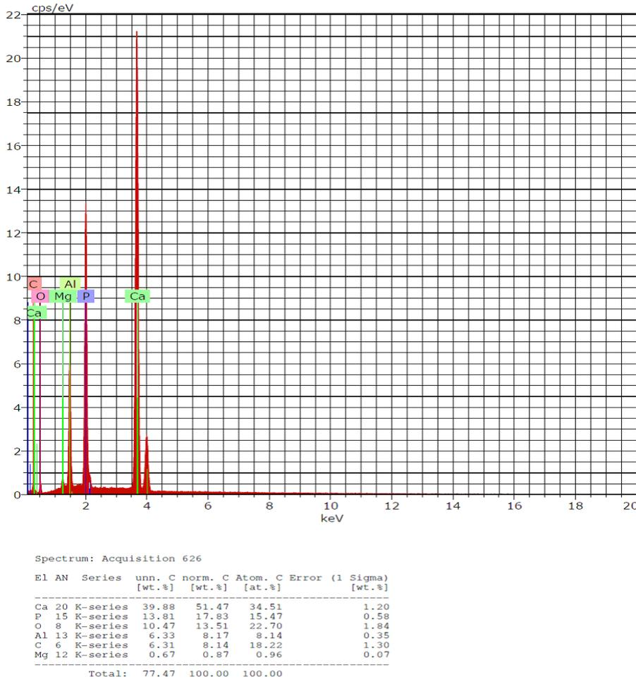
Figure 3. EDX of HA nanoparticles
