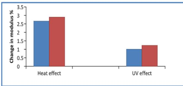
**Fig. 10.** Shows the behaviour of modulus elasticity when ageing for seventy two hrs victimisation heat at 37°C and ultraviolet
