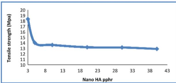
Fig. 5b). Effect of high quantities of nano HA on tensile strength of recipe
