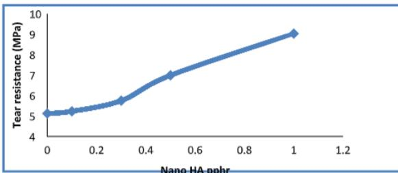
Fig. 6. Effect of nano HA on tear resistance of recipe
