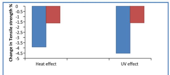
Fig. 8. Shows the behaviour of tensile strength after ageing for seventy two hrs victimisation heat at thirty seven°C and ultraviolet.
