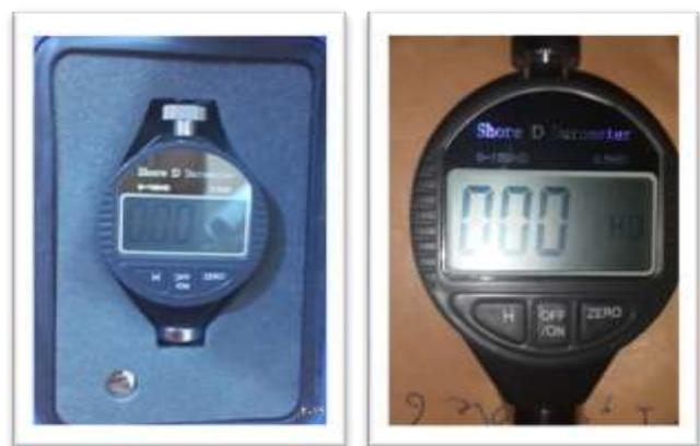
Figure 7. Hardness test instrument (Shore D)
