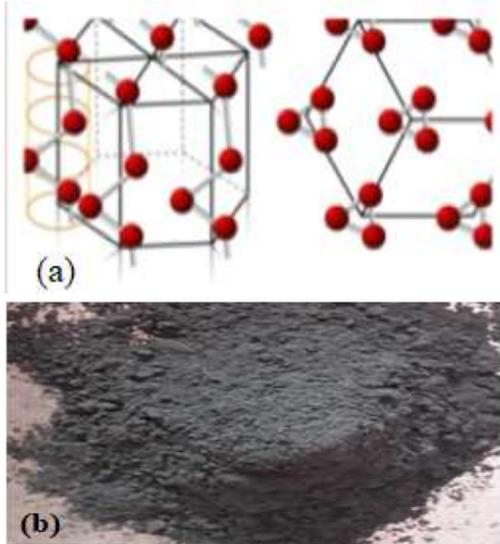
Figure 5. (a) Tellurium structure and (b) appearance [24]
