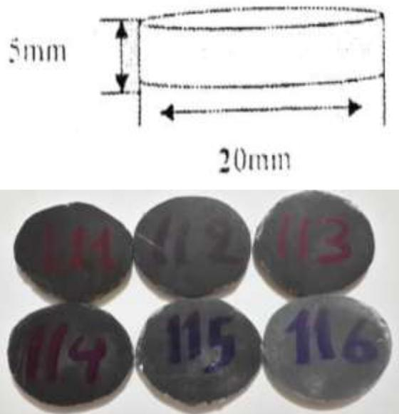
Figure 6. Hardness Samples Test
