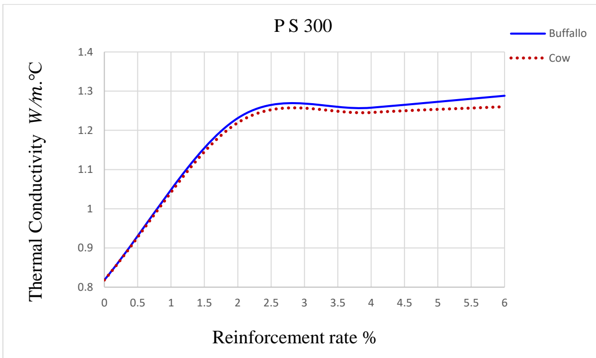
Scheme 6. The thermal Conductivity of the specimens opposite the reinforcement rates
