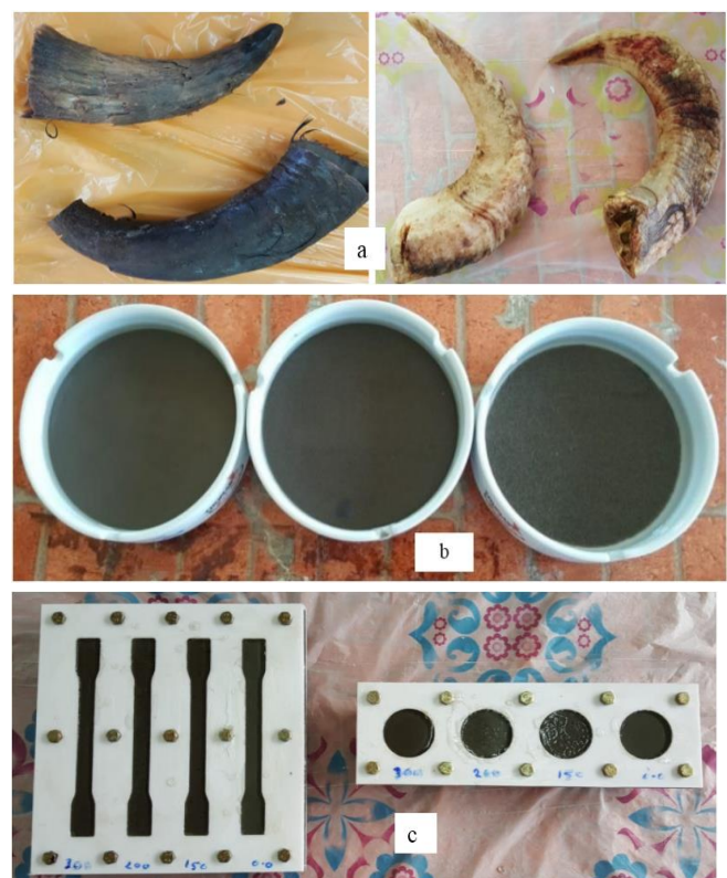
Scheme 1. a) Cows and buffalo horns, (b) the powder of horns (c) the Teflon molds
