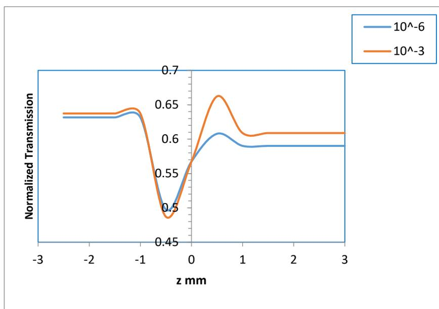
Figure 5. Z-Scan close-aperture data in two different concentrations of compounds (h) as liquid
