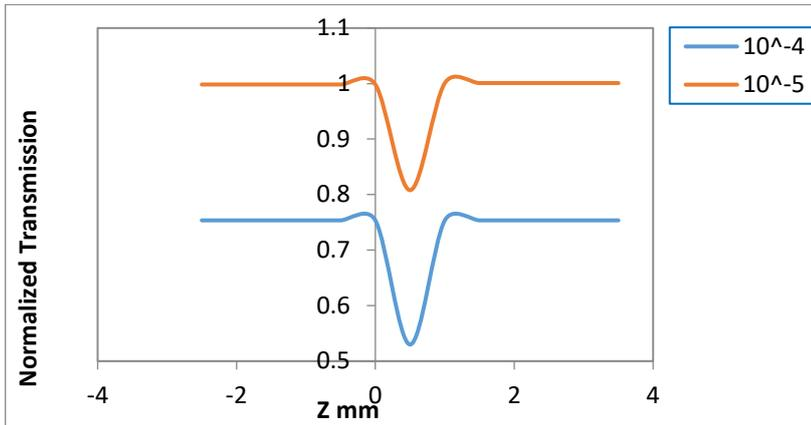
Figure 6. The Z-Scan data open-aperture of two verities concentration of compounds (h) as solution
