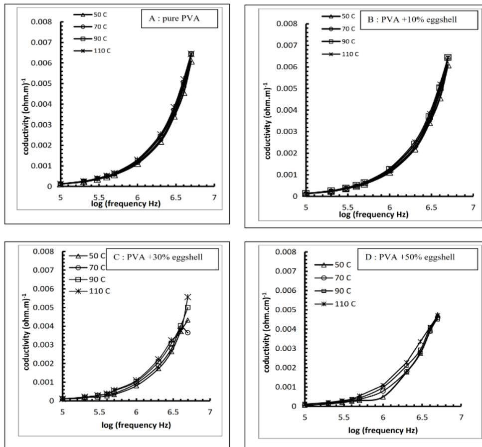
Figure 6. (A,B,C,D): Variation of AC conductivity with temperature for different additives of eggshells powder
