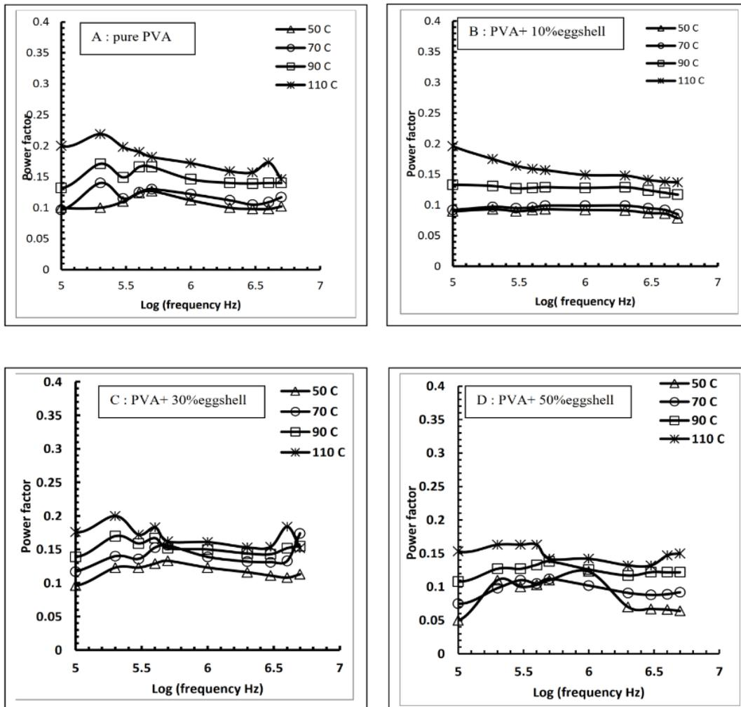
Figure 5. (A, B, C, D): Variation of power factor with temperature for different additives of eggshells powder
