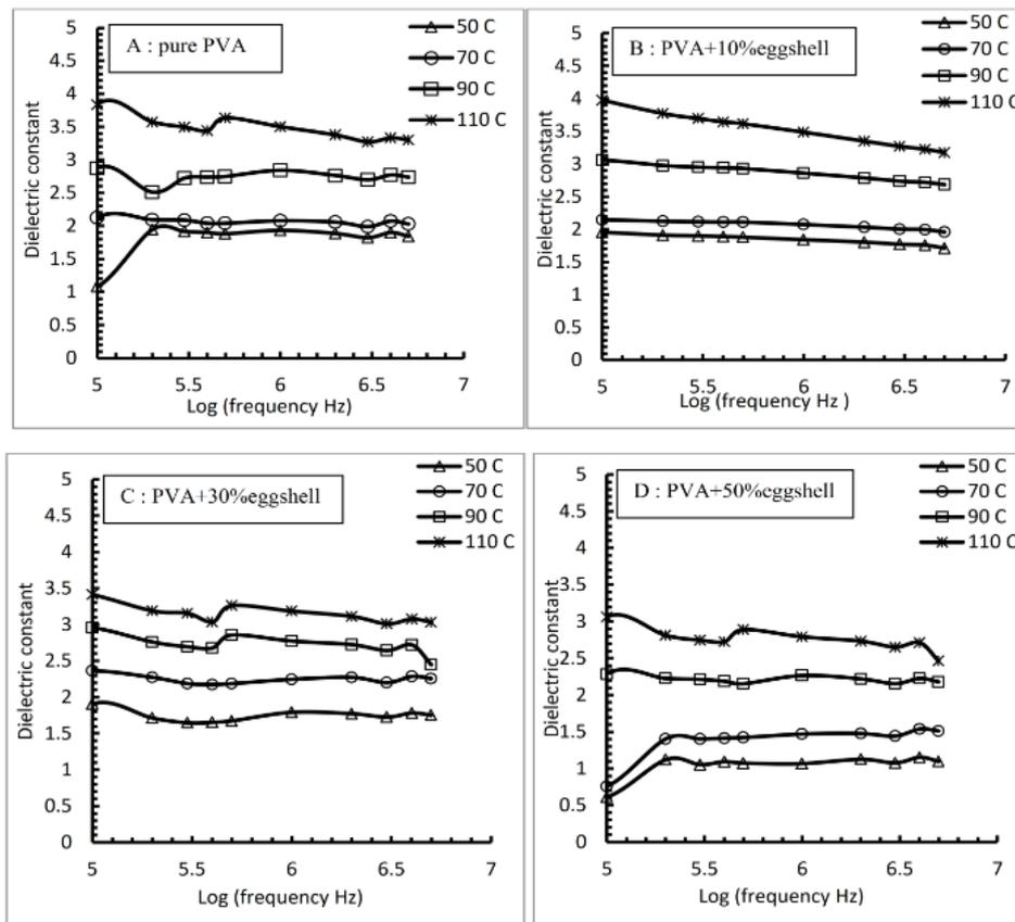
Figure 4. (A, B, C, D): Variation of dielectric constant with temperature for different additives of eggshells powder
