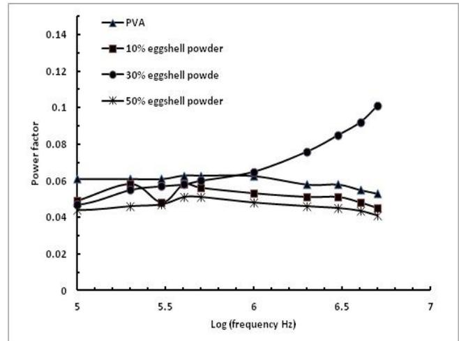
Figure 2. Power factor plot of PVA/eggshell powder composites at different frequencies and filler concentrations
