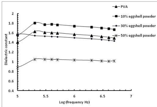
Figure 1. Dielectric constant plot of PVA/eggshell powder composites at different frequencies and filler concentrations
