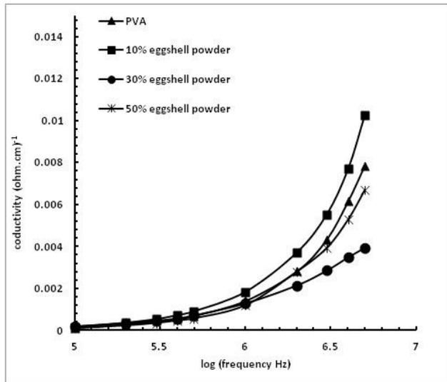
Figure 3. Electrical conductivity plot of PVA/eggshell powder composites at different frequencies and filler concentrations
