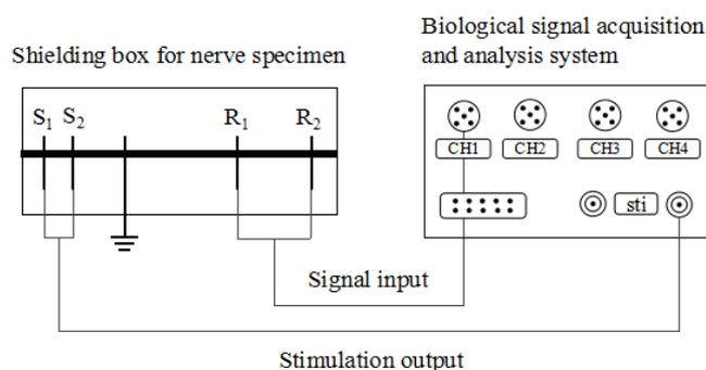
Figure 1. The schematic diagram of the experimental device. It is comprised of a nerve specimen shielding box and biological signal acquisition and analysis system. S1 and S2 are used as stimulating electrodes and R1 and R2 as recording electrodes. The middle wire is grounded to filter stimulus artifact.
