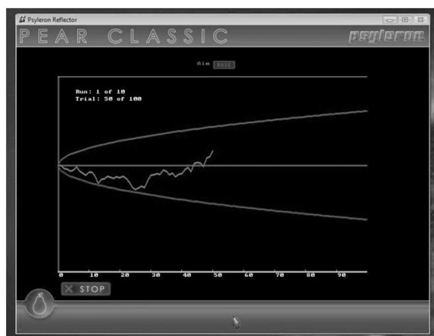
Figure 2. Screenshot of Reflector software collecting data from REG device; jagged center line is the moving cumulative deviation.
