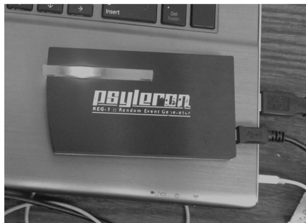
Figure 1. Random event generator (REG); Psyleron REG-1 device used throughout the following experiment.
