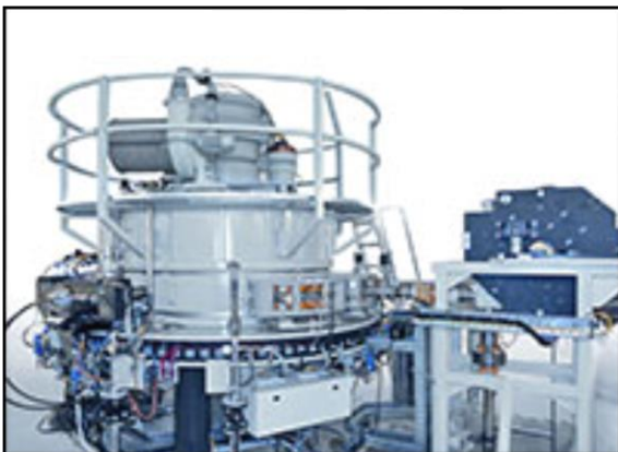
Figure 1. X-ray machine used in food irradiation
