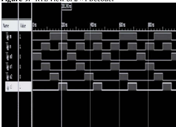
Figure 10. Output Waveform of 2 × 4 Decoder
