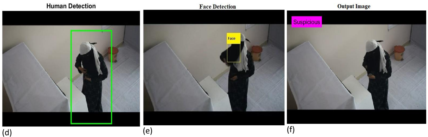
Fig. 5: Face Covered Recognition (a) input image (b) Detected customer and Score of input image, (c) NMS mask image, (d) human detection, (e) face detection, (f) output image (suspicious)
