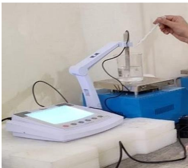
Fig: 2 An potentiometric cholesterol biosensor based on cholesterol oxidase NPs aggregates immobilized on CA membrane over the lower sensitive and of FIISE
