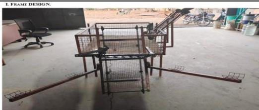
Fig. 3. Implementation of a garbage collection vessel robot
