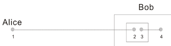
Figure 2. If it is possible to obtain entanglements larger than one of the initial states, then Alice and Bob could employ a scheme shown here to increase entanglement between distant parties by having Bob perform the Bell measurement on states 2 and 3, thereby creating a larger entanglement between 1 and 4 compared to the initial entanglement between 1 and 2.
