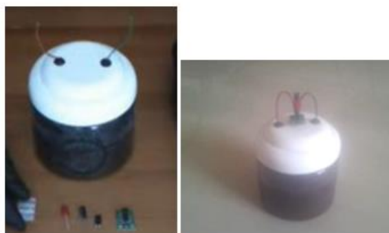
Fig. 4: Single chamber membrane less MFC unit (Generated by the Author)
