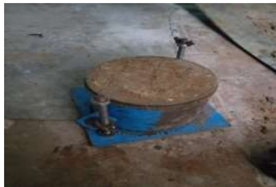
Figure 3.20 Sample of heavy compaction test with 0.8% Banana fibre
