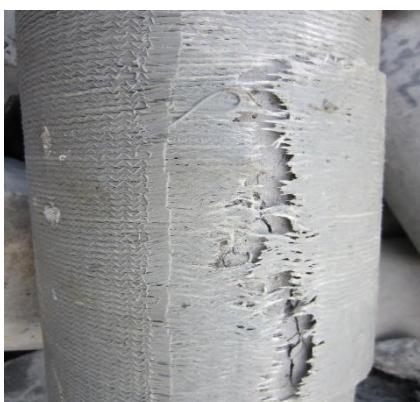
Figure 1. two sample of standard cylindrical screwed with glass and carbon FRP after test
