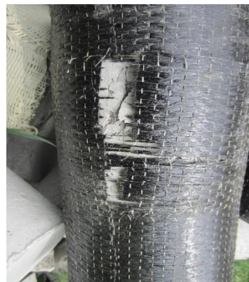
Figure 1. two sample of standard cylindrical screwed with glass and carbon FRP after test
