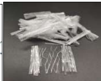
Fig3: Fibrillated Polypropylene fiber
