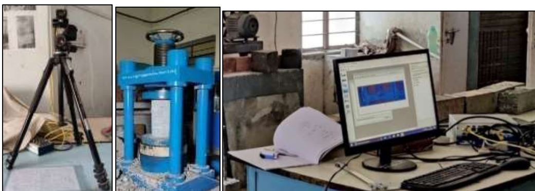
Fig 7: Use of Video Gauge Measurement Software for strain measurement in testing for modulus of elasticity of concrete
