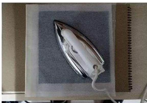
Figure 3. Fusing LDPE sheets by firmly pressing from the middle to the edges
