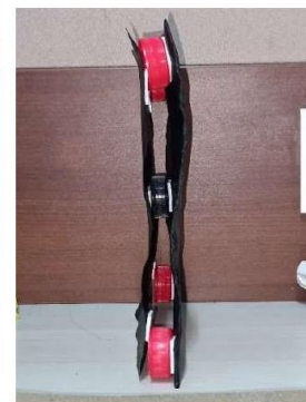
Figure 5. Bottle caps creating a cavity between the two layers
