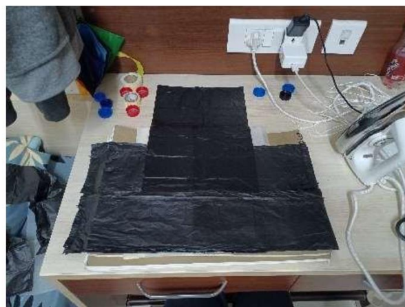
Figure 1. Unwrapped LDPE sheets placed in cross-laminated pattern
