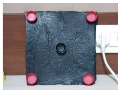
Figure 7. Bottle caps on fused LDPE sheets
