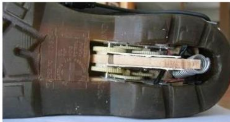
Figure 2- (b) View of arrangement in Power Generation shoe
