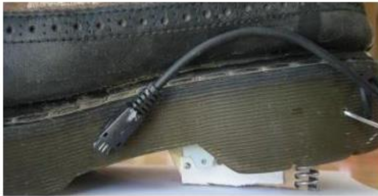
Figure 2- (a) View of arrangement in Power Generation shoe
