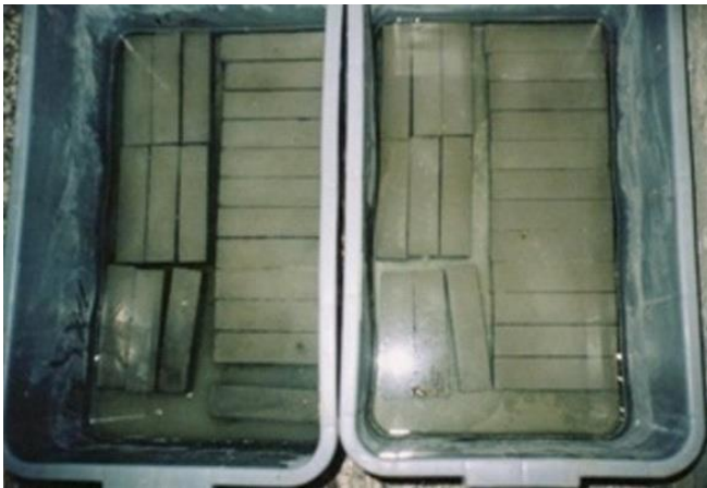
Figure.9 Specimen preservations in drinking water and aggressive water
