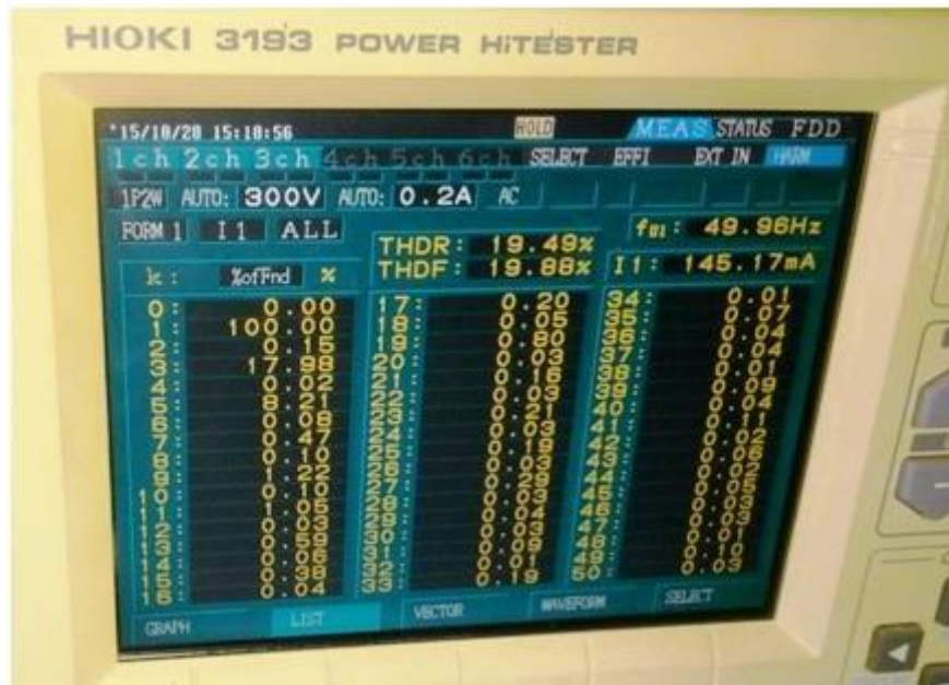
Figure 4 Power Analyzer Results of current harmonic (19.88%) using of MMC without filter
