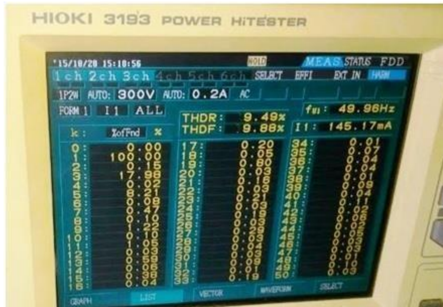
Figure 5 Power Analyzer Results of current harmonic (9.88%) using of MMC with filter
