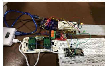
Figure 6: Initial Wiring conducted for testing using 5v power supply
