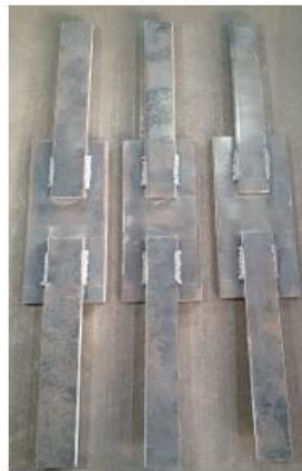
Figure 4. Welding was carried out on the coupons.
