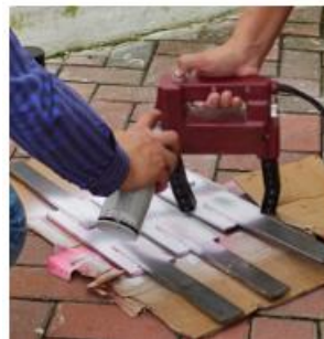
Figure 7. Magnetic particle inspection.
