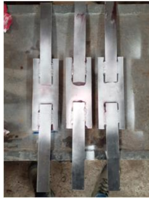
Figure 6. Inspection using penetrant inks.
