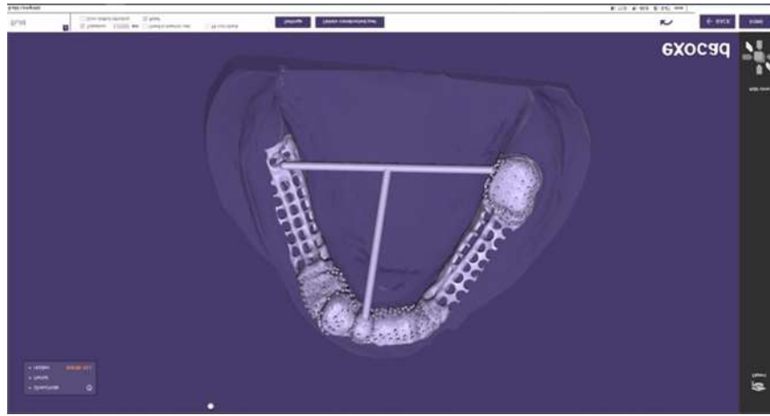
FIGURE 5: MANDIBULAR FRAMEWORK DESIGNING USING EXOCAD SOFTWARE
