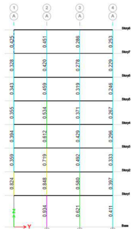
Figure 14. DCR value for Columns subjected to axial load at Grid Line 1.
