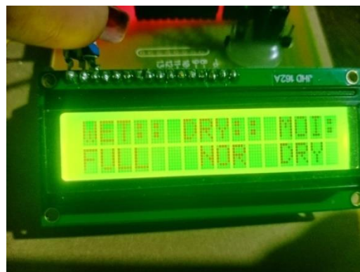
Fig 11: Message displayed that waste generated is Dry waste and wet dustbin is full
