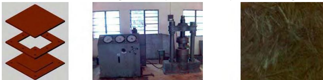
the placement of the mat is done alternatively with the pour of the resin. The setup of the experiment is as shown in Fig. 2.
