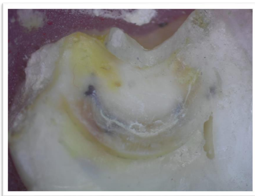
Figure (2): Adhesive mode of failure for the shear bond strength inspected under the stereomicroscope
