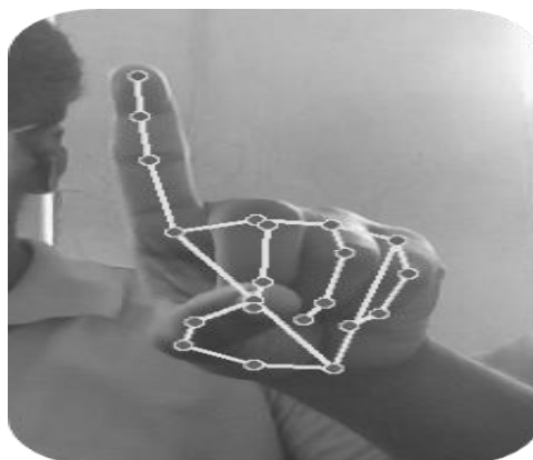
Fig. 7 Detecting Which Finger Is Up and Performing the Particular Mouse Function.
