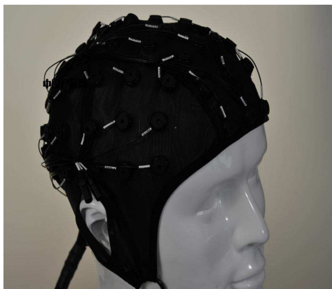
Figure 1. 64-lead Ag/AgCl cap
