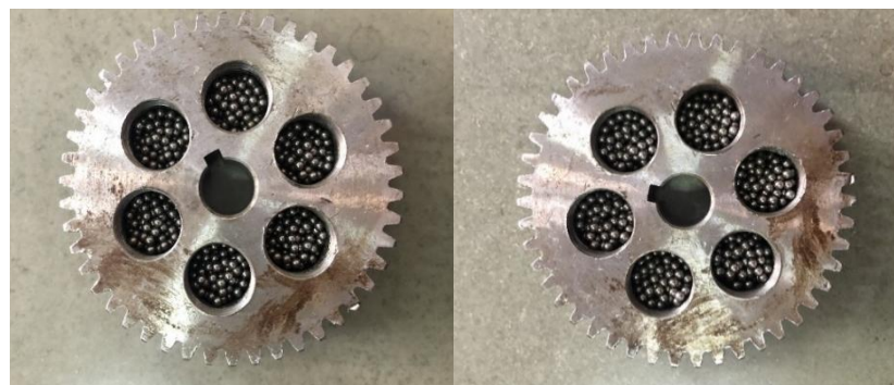
c) 50% Particle Filling Ratio
