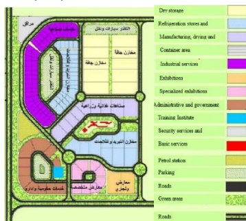
Fig 24 shows the indicative program for the various activities planned to be established in the logistics zone.[31]
