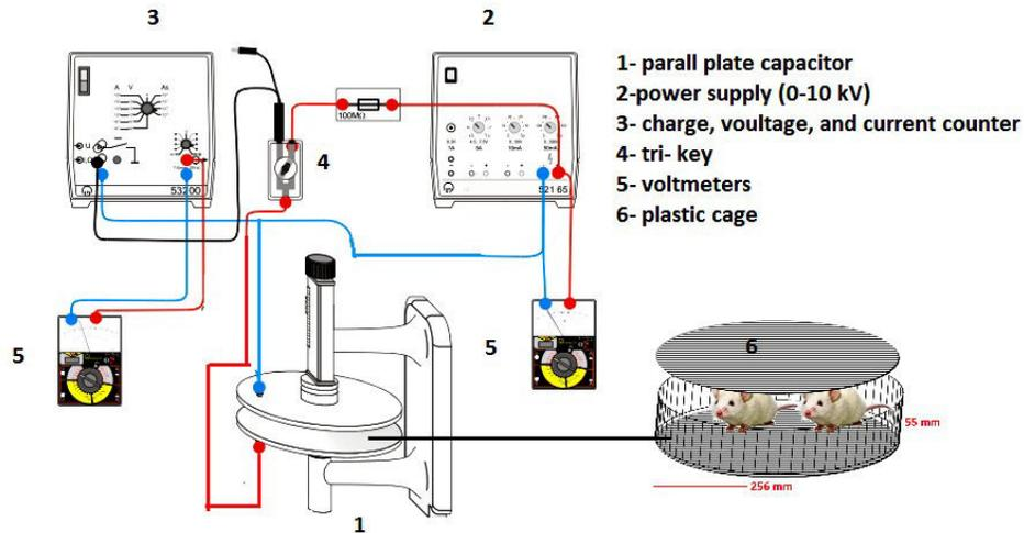
Fig. 1 shows the device for producing SEF. The input AC voltage was 220 V, and the output DC voltage was 0–10 kV where the SEF strength produced DC voltage was up to 160 kV generated between two parallel-electrode capacitors. The device comprised two plates separated by a distance within the range of 0–7 cm that was continuously adjustable, fine adjustment of the plate spacing of 1/10 mm intervals over a length of 2 mm, plate diameter of 255 mm, and plate thickness of 7 mm.
