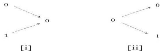
Figure 3. Landauer has shown that the irreversible computation, or the information erasure process, as in [i] yields an energy dissipation of kT \ln 2 and an entropy of k \ln 2 . The nondeterministic computation [ii] corresponds to the time-reversal process of [i].
