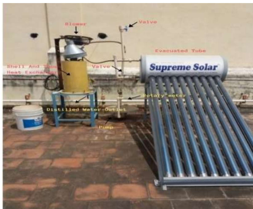
Figure 5 Experimental setup of evacuated tube collector driven humidification dehumidification system.
