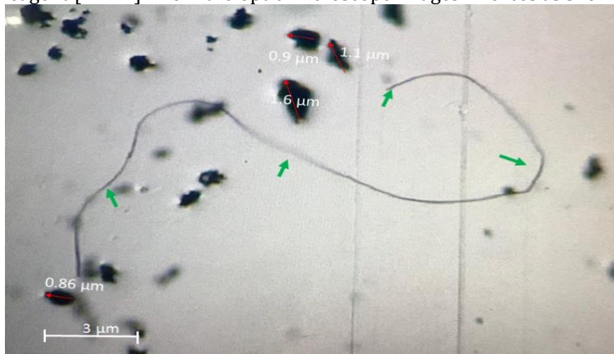
Figure 8. The optics images for graphite after oxidation in step 3 which precipitated after 1 h. to produce [Graphite-(O)x]
