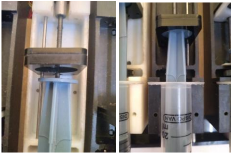
Fig. 9. The adjustment of syringe piston with the slider
