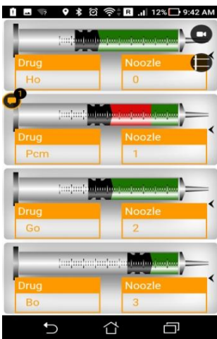
Figure 10. Red block will indicate the left out amount. (Injection of dose is completed).
