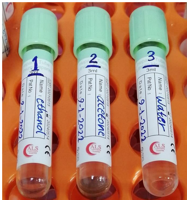
Fig. 1. The Colloidal of (Zn and ZnO) nanoparticles in ethanol, acetone and distilled water.
