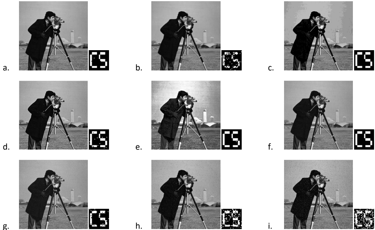
Fig. 7 Extracted watermark against image processing attacks on watermarked Cameraman image (a) Median filtering (b) Average filtering (c) JPEG Compression having QF=50 (d) Sharpening (e) Contrast enhancement (f) 5% Gaussian noise addition (g) 10% Gaussian noise addition (h) Salt and Pepper noise addition of 1% (i) Salt and Pepper noise addition 2%
