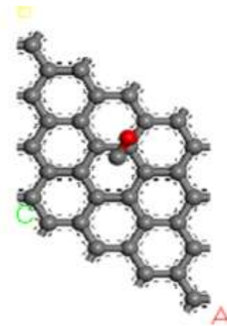
Figure (4) the graphene sheet adsorbed carbon monoxide with bond length and distance.
