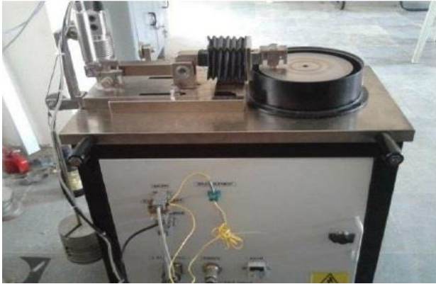
Figure 1. Pin-On-Disk wear testing apparatus
