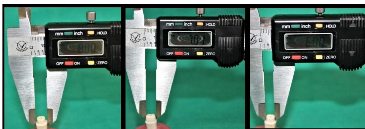
Figure 2 – Group A & B: Verification of 1 mm & 0.5 mm width with the help of digital vernier caliper
