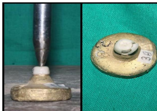
Figure 22- Application of load & fractured sample Universal testing machine controlled via a computer software program
