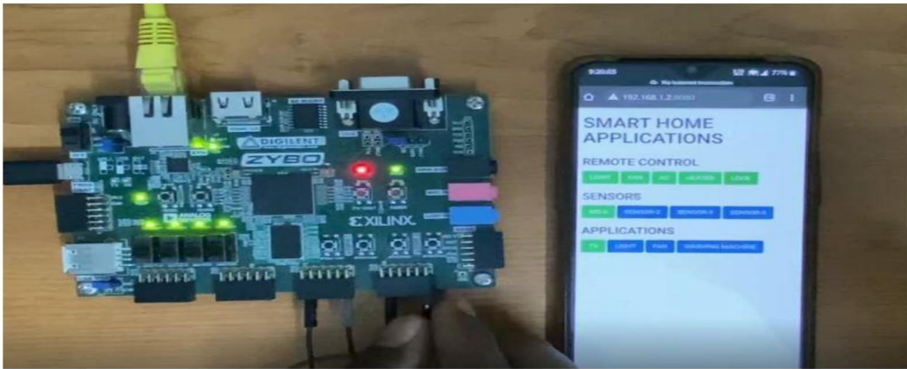
Fig.4 ZYBO control using webpage
