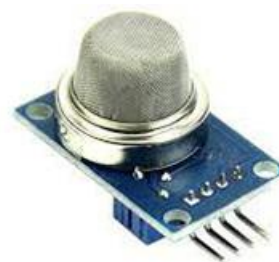
Fig .3: Gas Sensor.
