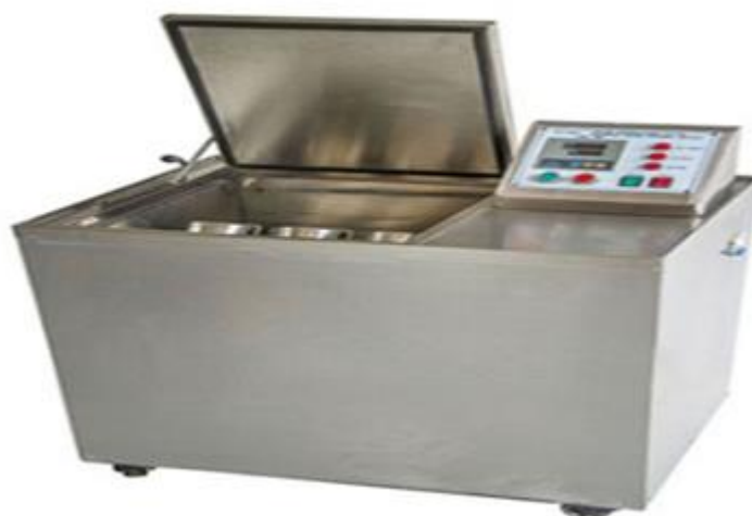
Figure 3 Colour fastness to washing tester.
