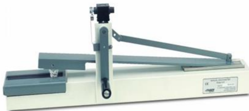
Figure 4 Rubbing fastness tester.
