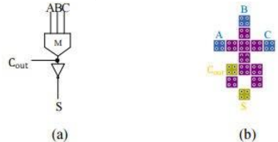
Fig. 4. One-bit approximate full adder: (a) schematic of AFA1, (b) layout of AFA1 in QCA.
