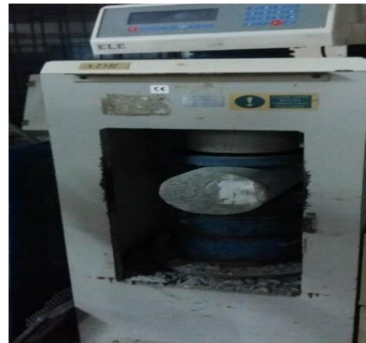
Fig. 2.10. Split tensile strength Test
