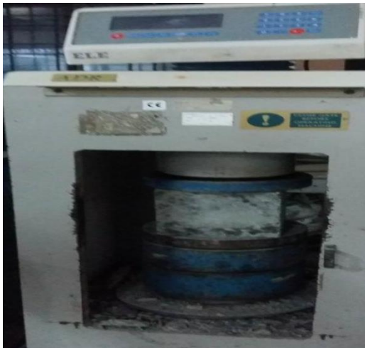
Fig. 2.9. Compressive Strength Test
